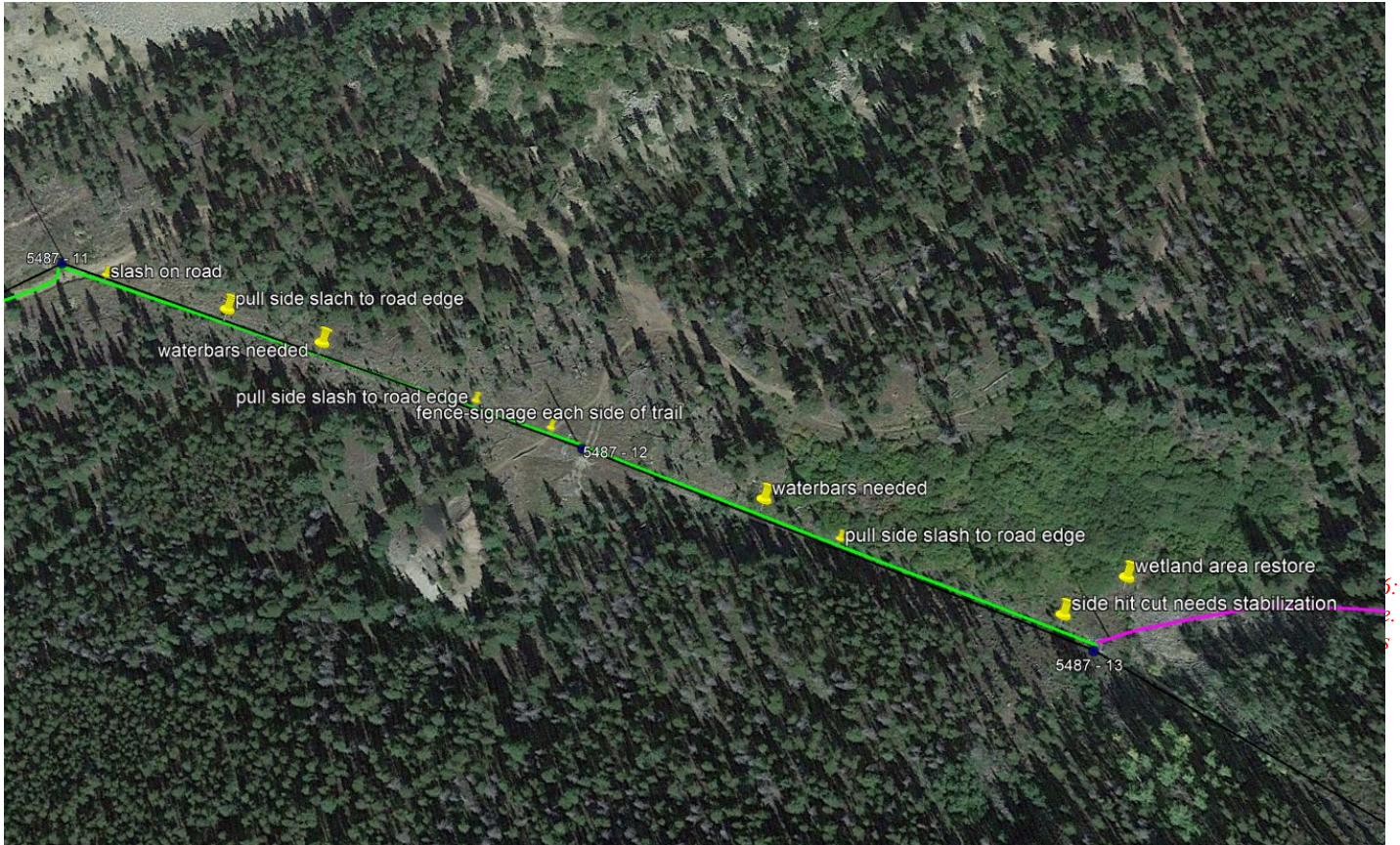
Figure 15, Transmission Line 5487 Restoration Site Map; Structures 11 through 13.
